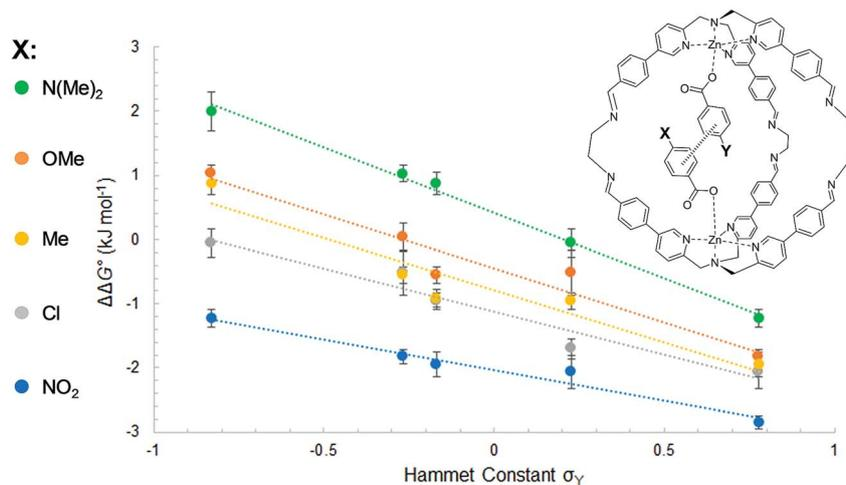
Fig. 4 Aromatic stacking energies ( $\text{kJ mol}^{-1}$ ) measured for the guest with substituent X (y-axis) plotted as a function of the Hammett constant  $\sigma_Y$  of the guest with substituent Y (x-axis). The slope and the  $R^2$  for each substituent are respectively NMe<sub>2</sub> ( $\rho = -2.0$ ,  $R^2 = 0.96$ ); OMe ( $\rho = -1.7$ ,  $R^2 = 0.99$ ); Me ( $\rho = -1.6$ ,  $R^2 = 0.91$ ); Cl ( $\rho = -1.3$ ,  $R^2 = 0.94$ ); NO<sub>2</sub> ( $\rho = -1.0$ ,  $R^2 = 0.96$ ).
