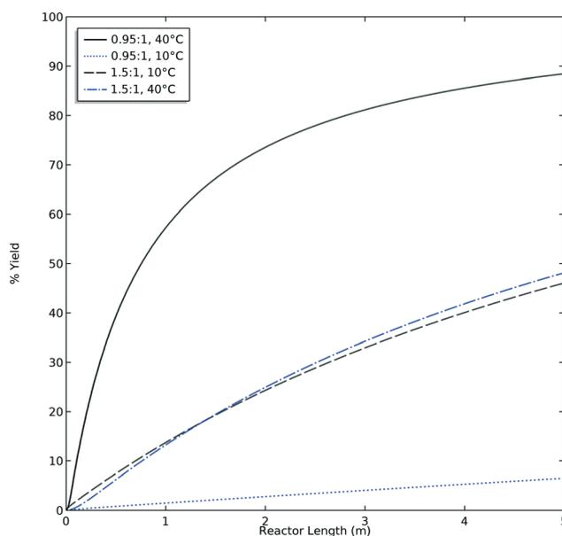
**Fig. 5** Theoretical product yield with respect to the limiting reagent as a function of reactor length at both high and low values of molar ratio and temperature predicted by CFD. Black and blue lines represent and 0.1 and  $1.0 \text{ ml min}^{-1}$  flow rates, respectively. Reaction condition: 5 m reactor with 1 mm ID.
