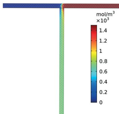
**Fig. 3** Three dimensional CFD mixing, without reaction, of  $1.5 \text{ mol m}^{-3}$  of both M4MAA (1) and DMF-DMA (2) entering a tee junction from left and right respectively and exit mixed downward.  $Pé$  and  $Re$  numbers for this simulation are  $1.51 \times 10^5$  and 5.02 respectively. Red and blue indicate high and low concentrations of DMF-DMA (2) respectively. The dashed line indicates where the reaction was assumed to initiate due to removal of the tee junction.
