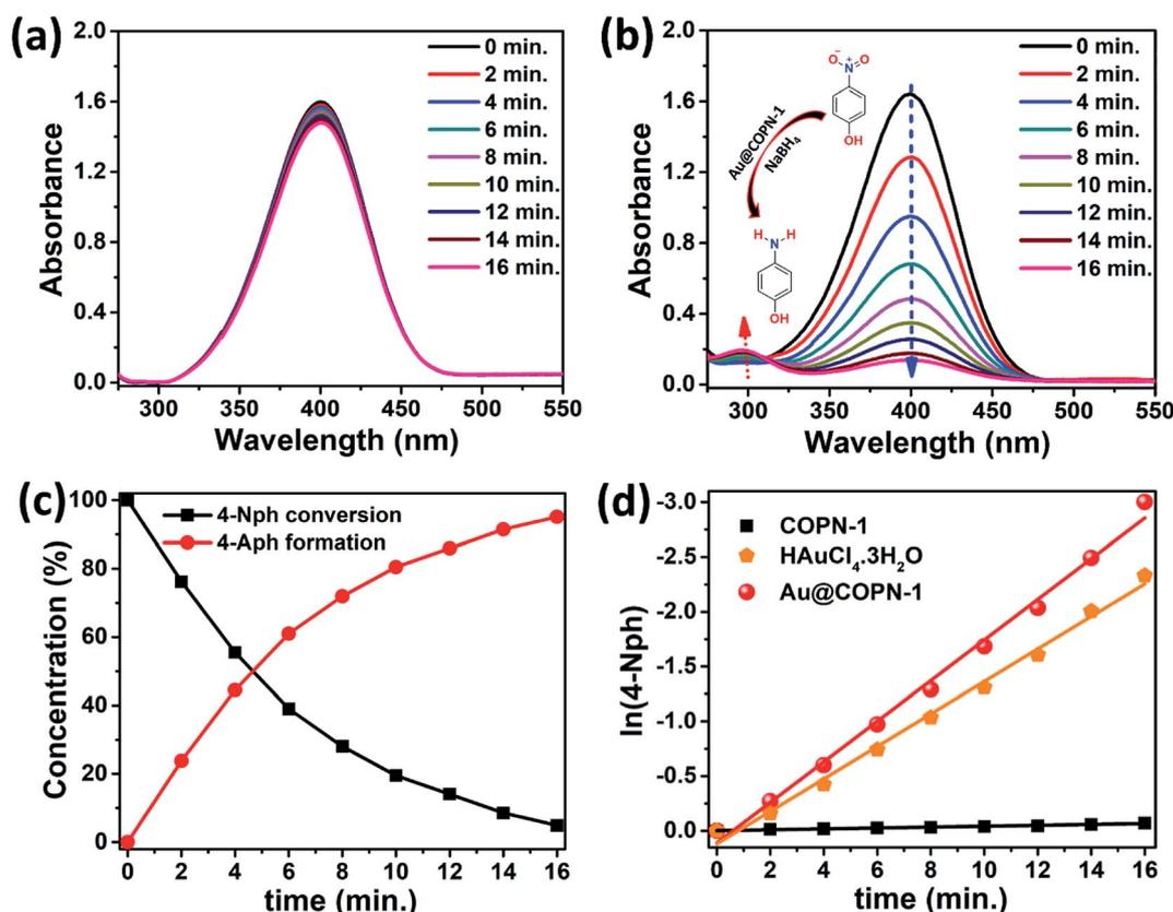
Fig. 5 Catalytic reduction of 4-nitrophenol by using  $\text{NaBH}_4$ , (a) COPN-1, (b) with Au@COPN-1 ( $4.6 \times 10^{-3}\text{ mM Au}$ ), (c) kinetics of reduction process of 4-Nph solution (4-Aph formation) and (d) fitted data of the pseudo-first-order kinetics (Au@COPN-1,  $\text{HAuCl}_4 \cdot 3\text{H}_2\text{O}$ , and COPN-1).
