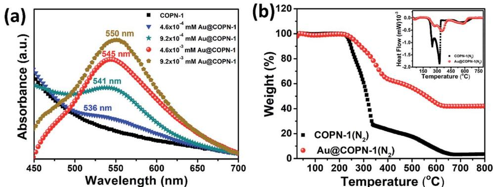
Fig. 4 (a) UV spectra of COPN-1 and Au@COPN-1 at different concentration ( $4.6 \times 10^{-4}$ ,  $9.2 \times 10^{-4}$ ,  $4.6 \times 10^{-3}$  and  $9.2 \times 10^{-3}$  mM Au) (b) TGA thermograms of COPN-1 and Au@COPN-1 ( $4.6 \times 10^{-3}$  mM Au) in  $\text{N}_2$ .
