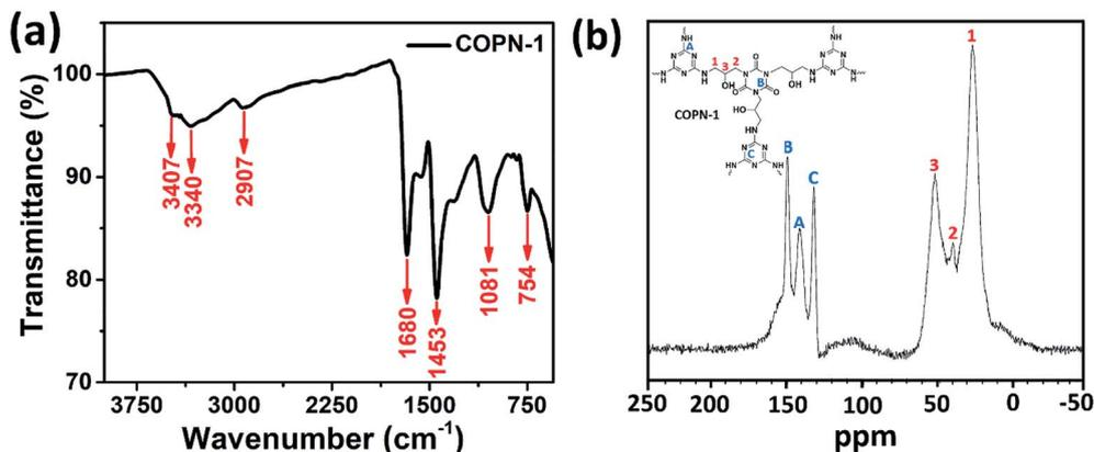
Fig. 1 (a) FTIR and (b) C-NMR spectra of COPN-1.
