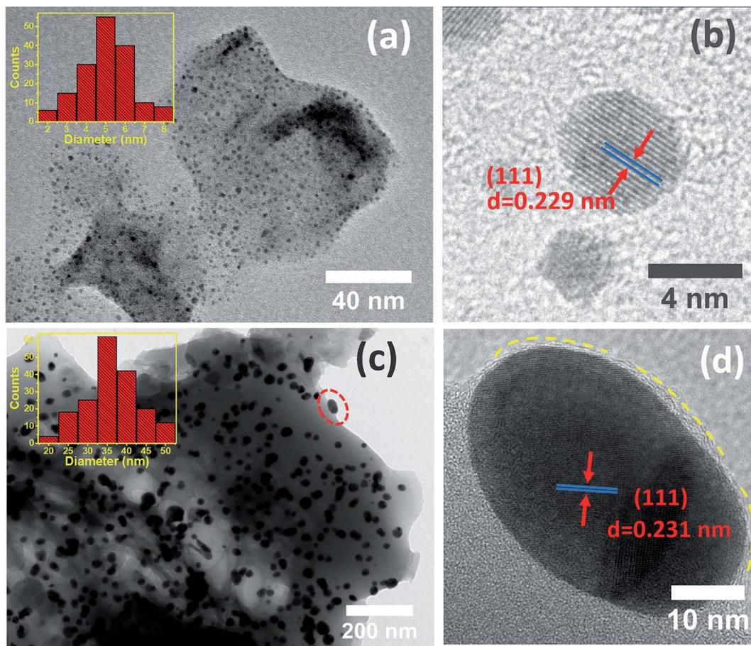
Fig. 3 (a and c) TEM images of Au@COPN-1 obtained from different concentrations of Au(+3) ( $4.6 \times 10^{-4}$  mM and  $4.6 \times 10^{-3}$  mM, respectively) with the corresponding particle size distribution histograms (b and d) The HR-TEM images of Au nanoparticles showing interplanar spacing.
