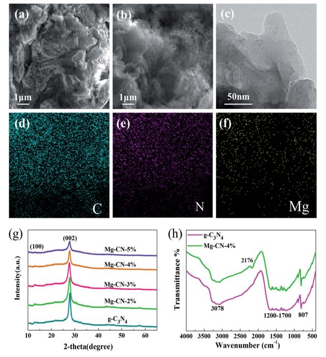
Fig. 1 SEM images of (a)  $g-C_3N_4$ , (b) Mg-CN-4%; (c) TEM image of Mg-CN-4%; (d) elemental mapping images of C, (e) N, (f) Mg of Mg-CN-4%; (g) XRD spectra of samples; (h) FTIR spectra of  $g-C_3N_4$  and Mg-CN-4%.
