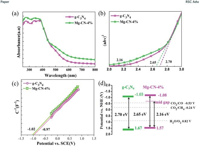
Fig. 3 (a) UV-vis diffuse reflectance spectra, (b) the plots of  $(ah\nu)^2$  versus  $h\nu$  for the band gap energies, (c) Mott–Schottky plots, (d) band gap structure of g-C<sub>3</sub>N<sub>4</sub> and Mg-CN-4%.
