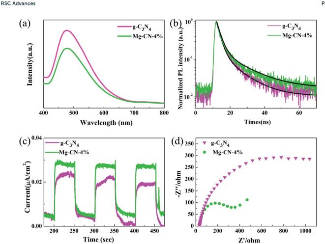
Fig. 4 (a) Photoluminescence spectra, (b) time-resolved PL spectra, (c) transient photocurrent-time curves, (d) electrochemical impedance spectra of g-C<sub>3</sub>N<sub>4</sub> and Mg-CN-4%
