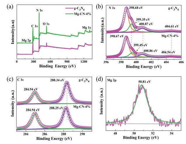
Fig. 2 (a) Wide survey scans, (b) N1s high-resolutions, (c) C1s high-resolutions of g-C₃N₄ and Mg-CN-4%, (d) Mg2p high-resolutions of Mg-CN-4%.
