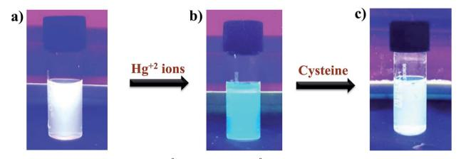
Fig. 6 Digital images of (a) WLEM; (b) WLEM with Hg<sup>2+</sup>; and (c) WLEM with Hg<sup>2+</sup> ions and Cys under UV light ( $\lambda_{ex} = 365 \text{ nm}$ ).
