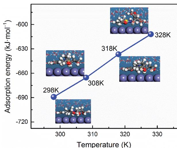
Fig. 10 Dependence of adsorption energy on the temperature for adsorbed AEM2 molecule on Fe(110).
