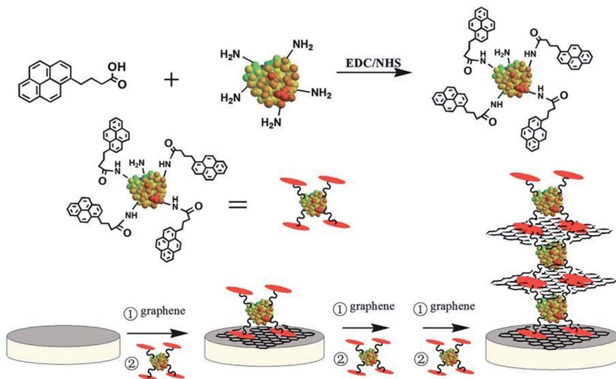
Fig. 5 Schematic illustration of the immobilization of GOx enzymes on graphene *via* pyrene and the subsequent fabrication of single- and multi-layered enzyme electrodes. [Reprinted with permission from ref. 196, J. Liu, N. Kong, A. Li, X. Luo, L. Cui, R. Wang and S. Feng, Graphene Bridged Enzyme Electrodes for Glucose Biosensing Application, *Analyst*, 2013, **138**, 2567–2575. Copyright© Royal Society of Chemistry.]
