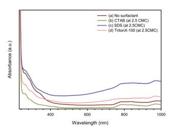
Fig. 4 UV adsorption spectra of PEDOT: PSS at the EDOT: PSS weight ratio of 1:11 and EDOT: Na<sub>2</sub>S<sub>2</sub>O<sub>8</sub> mole ratio of 1:2 using various surfactant types: (a) no surfactant, (b) CTAB (at 2.5CMC), (c) SDS (at 2.5CMC), and (d) Triton X-100 (at 2.5CMC).
