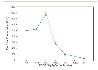
Fig. 9 Electrical conductivity of PEDOT: PSS at the EDOT: PSS weight ratio of 1:11 and at various EDOT: Na<sub>2</sub>S<sub>2</sub>O<sub>8</sub> mole ratios.
