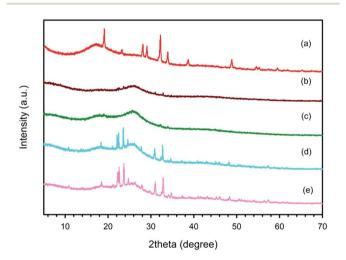
Fig. 3 XRD spectra of commercial PSSNa and PEDOT:PSS at the EDOT: PSS weight ratio of 1:11 and at various EDOT: Na<sub>2</sub>S<sub>2</sub>O<sub>8</sub> mole ratios: (a) PSSNa, and EDOT:  $Na_2S_2O_8$  mole ratio of (b) 1:1, (c) 1:2, (d) 1:3 and (e) 1:4.
