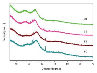
Fig. 2 XRD spectra of PEDOT:PSS at the EDOT: Na<sub>2</sub>S<sub>2</sub>O<sub>8</sub> mole ratio of 1:1 and at various EDOT: PSS weight ratios: (a) EDOT: PSS weight ratio of 1:1, (b) EDOT: PSS weight ratio of 1:5, (c) EDOT: PSS weight ratio of 1:11, and (d) EDOT: PSS weight ratio of 1:13.
