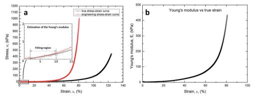
Fig. 4 (a) Stress—strain curves of the PVA scaffold obtained from compression test. (b) Evolution of the Young's modulus as a function of true strain. The values of the Young's modulus were calculated from the true stress—strain data. The graph shows marked non-linear trend of the Young's modulus.
