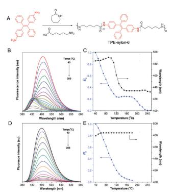
Fig. 17 (A) Synthetic route of TPE-nylon-6. (B) Fluorescence spectra of (B) TPE-nylon-6 and (D) TPE-doped nylon-6 at different temperatures. Plots of relative fluorescence intensity ( $I/I_0$ ) and emission wavelength of (C) TPEnylon-6 and (E) TPE-doped nylon-6 versus temperature, where  $I_0$  is fluorescence intensity at 40 °C. Reproduced from ref. 84 with permission from Wiley-VCH.
