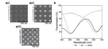
Fig. 1 Comparison of mono- and bimetallic LSPR sensors. (a) SEMs showing (i) monometallic Al, (ii) monometallic Au, and (iii) bimetallic Al/ Au regions. (b) Transmission response of arrays of Al-only (dotted-blue), Au-only (dotted-red), and bimetallic Al/Au (black solid) in water.
