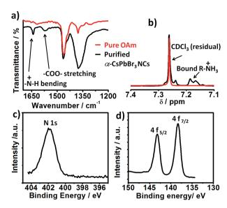
Fig. 2 (a) FTIR spectra of the purified CsPbBr $_3$  NCs (black) compared to pure oleyl amine (red). (b)  $^1$ H NMR of purified  $\alpha$ -CsPbBr $_3$  NCs in CDCl $_3$  (black) (c) XPS N 1s and (d) Pb 4f core level XPS spectra CsPbBr $_3$  NCs
