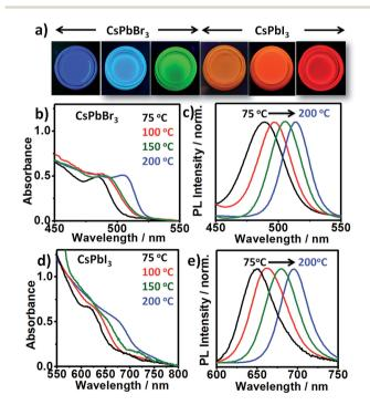
Fig. 4 (a) UV illuminated photographs of colloidal solutions of different sized  $CsPbX_3$  NCs (X = Br, I). Absorption (b) and emission spectra (c) of  $CsPbBr_3$  NCs at different reaction temperatures (75–200 °C). Absorption (d) and emission spectra (e) of  $CsPbI_3$  NCs at different reaction temperatures (75–200 °C).
