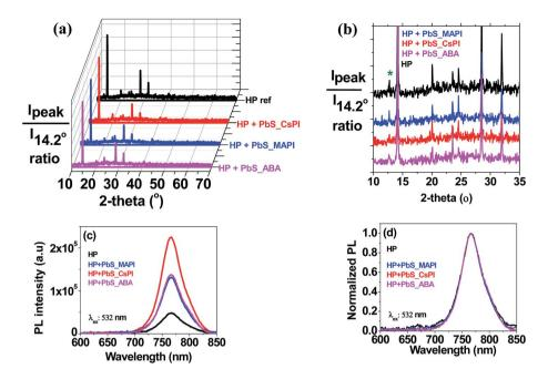
Fig. 2 Crystallographic and optical characterization of perovskite films without (HP) and with PbS QDs (50  $\mu$ g ml<sup>-1</sup>) deposited on glass of PbS QDs with the different capping ligands including MAPI, CsPI and 4-aminobenzoic acid (ABA). XRD spectra (a) and a zoom-in from 10 to 35° (b) (the \* symbol indicates the PbI<sub>2</sub> diffraction peak); (c) photoluminescence (PL) and (d) normalized PL spectra.
