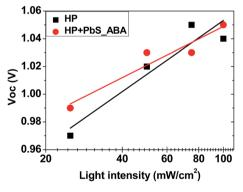
Fig. 5 Dependence of open circuit voltage on light intensity for the champion cells (see Table 2) with the architecture FTO/SnO<sub>2</sub>/ absorber/spiro-OMeTAD/Au, in which absorber layers were perovskite films without (HP) and with PbS QDs (50  $\mu$ g ml<sup>-1</sup>) and PbS QDs had the 4-aminobenzoic acid (ABA) ligand. The measurement was done at room temperature.
