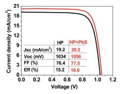
Fig. 4 Photovoltaic characteristics of the best FTO/SnO<sub>2</sub>/absorber/ spiro-OMeTAD/Au solar cells, in which absorber layers were perovskite films without (HP) and with PbS QDs (50 µg ml<sup>-1</sup>) and PbS QDs had the 4-aminobenzoic acid (ABA) ligand
