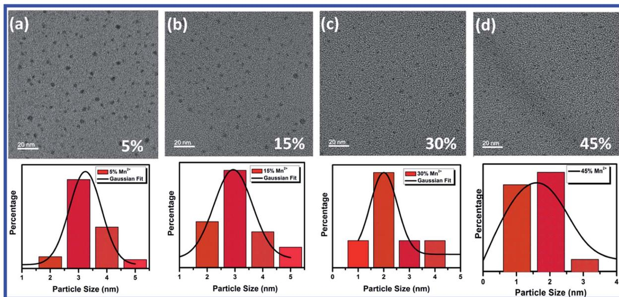
Fig. 4 TEM characterization of  $\text{CH}_3\text{NH}_3\text{Pb}_{1-x}\text{Mn}_x\text{I}_3$  PQDs with different  $\text{Mn}^{2+}$  concentration and their corresponding statistical analysis graph of particle size distribution (a) 5% with average particle size 3.5 nm, (b) 15% with average particle size 3 nm, (c) 30% with average particle size 2 nm, and (d) 45% with average particle size 1.5 nm.
