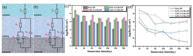
Fig. 8 (a) The electrical equivalent circuit models of stage I; (b) the electrical equivalent circuit models of stage II; (c) coating resistance ( $R_c$ ); (d) charge transfer resistance ( $R_{\rm ct}$ ), respectively.
