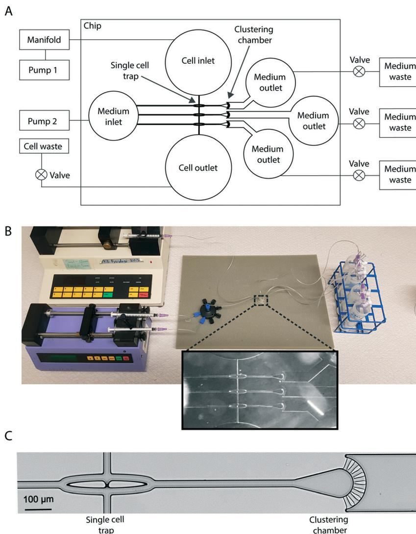
**Fig. 1** Schematic illustration of the system and the microfluidic chip. (A) Overview of the CAGE chip and its connections to the other system components (pumps, valves, and manifold). (B) Picture of the setup. The inset shows a magnification of the central part of the CAGE chip. (C) Image showing one of the single-cell traps in the CAGE chip together with the corresponding clustering chamber, with its eight outward radiating fluidic channels present in the fan-shaped cell restrainer.
