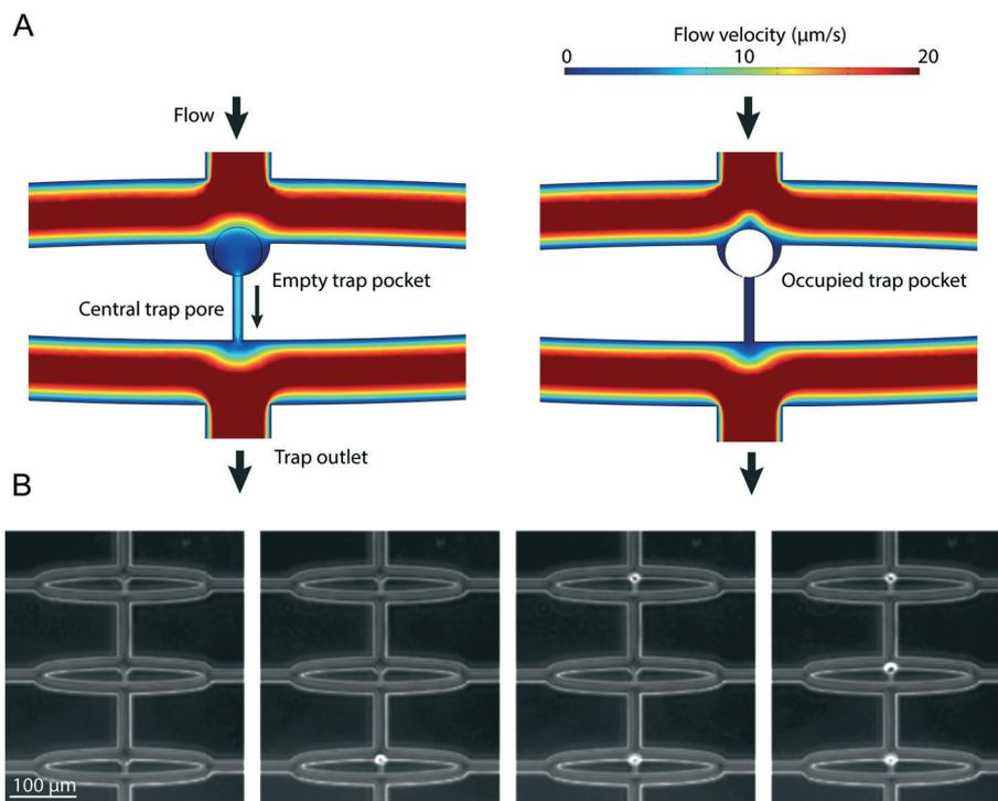
**Fig. 2** Overview of flow dynamics and operation of the single-cell trap. (A) FEM simulation of the flow velocities ( $\mu\text{m s}^{-1}$ ; color-coded) in and around the hydrodynamic single-cell trap with an empty (left) or occupied (right) trap pocket. Occupation of the trap prevents fluid flow through the centrally located trap pore. (B) Image sequence showing the trapping of three individual cells in the three serially connected traps.
