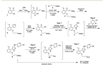
Scheme 2 Continuous manufacturing production route for prexaseratib monolactate monohydrate under cGMP conditions. 112 Reprinted with permission from AAAS.
