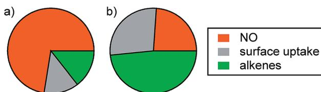
Fig. 7 Relative contribution of the three sinks to  $O_3$  loss in the environmental chamber under (a) post-cooking and (b) background conditions. The contribution of alkenes is determined based on the  $O_3$  loss that is not accounted for by the other two processes.
