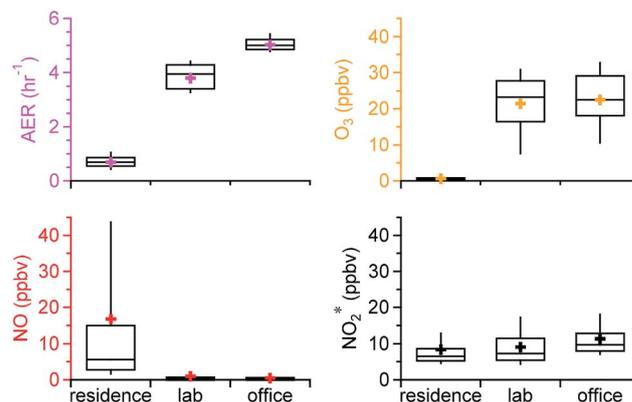
Fig. 1 Statistics of the air exchange rate (AER) and mixing ratios of O<sub>3</sub>, NO, and the sum of NO<sub>2</sub> and HONO (NO<sub>2</sub>\*) observed in three indoor environments in Syracuse, NY, over the entire field study period. The box and whisker plots show the median (line), mean (marker), upper and lower quartiles (box), and the 10th and 90th percentiles (whiskers).
