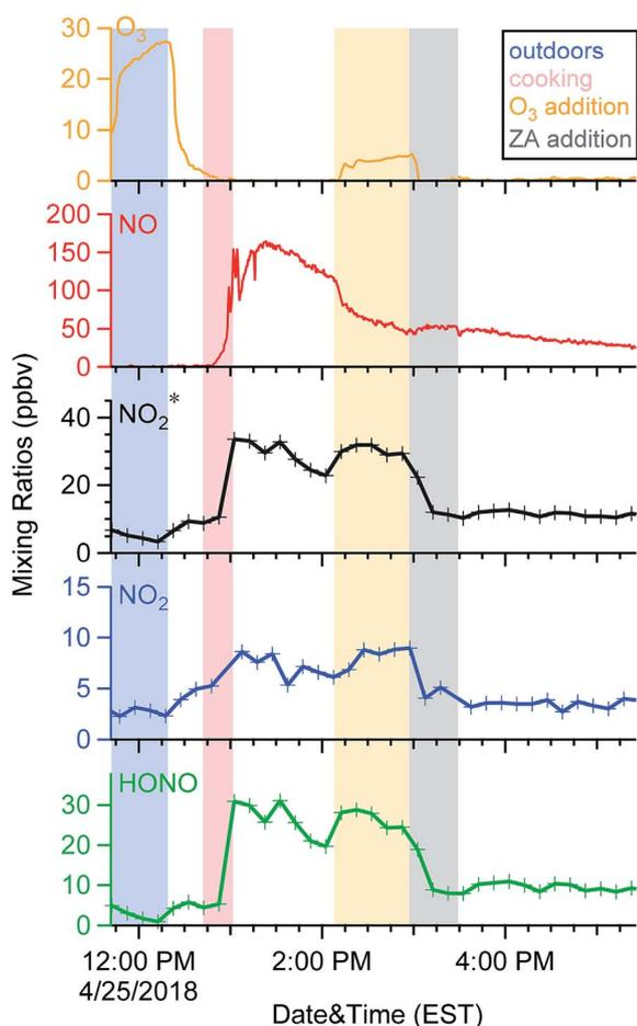
Fig. 6 Time series of oxidant\* observed in the residence sampled through the environmental chamber during an  $\text{O}_3$ -perturbation experiment performed after cooking. Shaded areas indicate different conditions noted in the legend of the graph.
