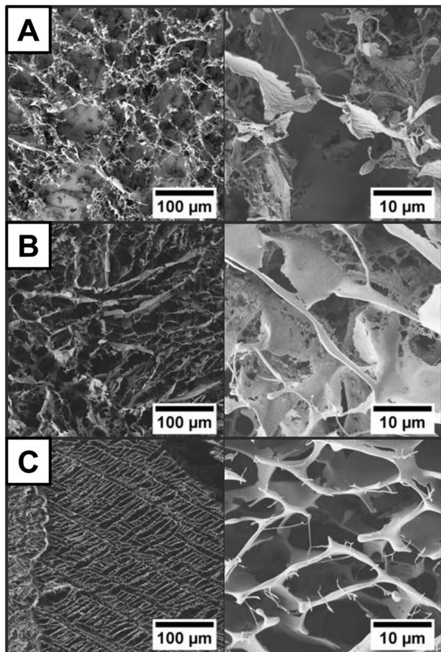
Fig. 3 SEM images of different CdSe NPL cryoaerogel coatings. The concentration of Cd<sup>2+</sup> in the original aqueous NPL solutions increases from panel A to C (A: 10 mM, B: 28 mM, and C: 70 mM). For the preparation of each sample, 20 μL of the respective NPL solution was used. The KOH concentration was kept constant at  $1 \times 10^{-2}$  M.
