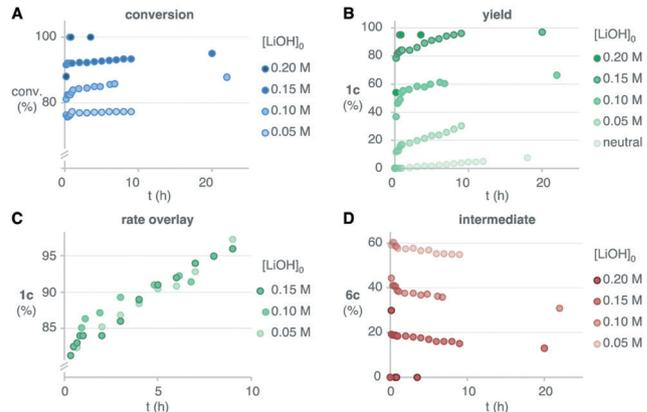
**Scheme 5** Effect of the initial concentration of base additive in the conversion, yield and accumulation of endoperoxide intermediate. Percentages are relative to the initial concentration of the limiting diketone **4c** (0.05 M).
