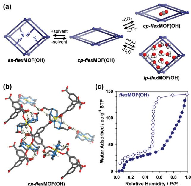
Fig. 5 (a) Schematic illustration of the phase transitions of *flexMOF(OH)* upon guest removal/reintroduction and adsorption/desorption of CO<sub>2</sub> and H<sub>2</sub>O molecules. (b) Hydrogen bonds of *cp-flexMOF(OH)* as represented by dotted lines, and (c) its water vapour isotherm at 298 K. Filled and empty circles represent adsorption and desorption curves, respectively.
