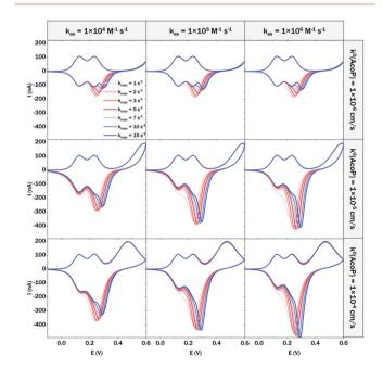
Fig. 10 Modelling of the CVs showing the influence of three different constants, the heterogeneous electron transfer constant of AcoP ( $k^0$ ), the kinetic rate constant of the complex formation ( $k_{as}$ ) and the constant of the intermolecular electron transfer within the complex ( $k_{inter}$ ), on the shape of the simulated voltammograms at 20 mV s<sup>-1</sup> (capacitive current is excluded).
