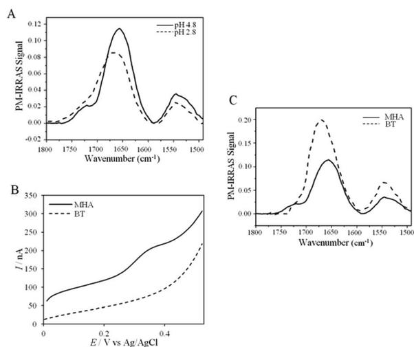
Fig. 5 AcoP behavior on SAMs. (A) PMIRRAS spectrum of AcoP at  $20\text{ }\mu\text{M}$  adsorbed for 1 h on MHA-Au in  $10\text{ mM NH}_4\text{AC}$  at pH 4.8 (solid line) and pH 2.8 (dashed line); (B) SWVs of AcoP adsorbed on MHA (solid line) or BT (dashed line) in  $10\text{ mM NH}_4\text{AC}$  at pH 4.8; (C) PMIRRAS spectra of AcoP at  $20\text{ }\mu\text{M}$  in  $10\text{ mM NH}_4\text{AC}$  at pH 4.8 adsorbed for 1 h on MHA-Au (solid line) or BT-Au (dashed line).
