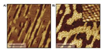
Fig. 3 STM images of (A) 0.06 ML and (B) 0.19 ML trifluoroacetate on Au(110) demonstrate that carboxylates form dense local island at low global coverages; scale bar, 10 nm, sample bias: 0.5–1.5 V, tunneling current: 0.1 nA. Inset in B reveals the  $c(2\times2)$  ( $\sim$ 400 K annealed surface in B).
