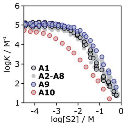
Fig. 16 Association constants ( $\log K/\text{M}^{-1}$ ) for formation of the **6**·**13** complex as a function of alcohol concentration (S2) in *n*-octane (S1) at 298 K. Data highlighted are 1-octanol **A1** (black), 3-ethyl-3-pentanol **A9** (blue) and trifluoromethyl-2-octanol **A10** (red).
