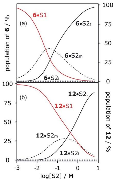
Fig. 13 Speciation of two different H-bond acceptors (A) in mixtures of 1-octanol (S2) and *n*-octane (S1). (a) **6** ( $\beta = 10.7$ ). (b) **12** ( $\beta = 7.8$ ). A·S1 solid red lines; A·S2<sub>m</sub> dashed lines; A·S2<sub>i</sub> dotted lines; A·S2<sub>t</sub> solid black lines. Calculated using the following H-bond parameters for S2:  $\alpha_i = 0$ ,  $\alpha_t = 3.5$ ,  $\alpha_m = 2.7$  and  $\beta_i = 5.3$ ,  $\beta_t = 6.9$ ,  $\beta_m = 5.3$ .
