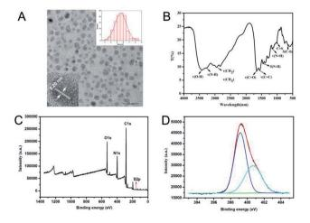
Fig. 2 TEM image (A), FTIR spectrum (B), XPS survey spectrum (C), and high-resolution XPS survey of N1s (D) of N-CDs. Insets of (A) are the HRTEM (left) and size distribution (right) of N-CDs.
