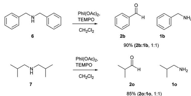
Scheme 4 Comparative study on symmetrical secondary amines. Reaction conditions unless otherwise specified: amine 1 (1 equiv.),  $\text{PhI}(\text{OAc})_2$  (1 equiv.), TEMPO (0.1 equiv.), anhydrous  $\text{CH}_2\text{Cl}_2$ , 0 °C to rt, 20 min.
