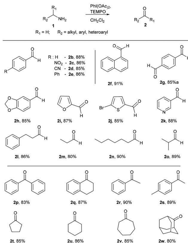
Scheme 2 Oxidation of primary amines to aldehydes and ketones. Reaction conditions unless otherwise specified: amine **1** (1 equiv.), PhI(OAC)<sub>2</sub> (1 equiv.), TEMPO (0.1 equiv.), 0 °C to rt, 20 min, anhydrous CH<sub>2</sub>Cl<sub>2</sub>. <sup>a</sup>PhI(OAC)<sub>2</sub> (2 equiv.), TEMPO (0.2 equiv.).
