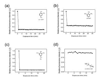
Fig. 4 Changes in the relative fluorescence intensities  $(I_x/I_i)$  of 1:2 TPE-CMP (0.375 mg mL<sup>-1</sup> in CH<sub>2</sub>Cl<sub>2</sub>) upon various exposure time in the presence of (a) 2,4-DNT, (b) 2,6-DNT, (c) PA, and (d) 2,3-DN-2,3-DM. [Explosives] =  $2.5 \times 10^{-3}$  M. Excitation wavelength 330 nm.  $I_i$  and  $I_x$  represent fluorescence intensity at 550 nm in the absence and presence of explosives, respectively.
