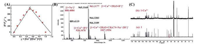
Fig. 7 (A) Job's plot for the complexation of 1 with  $Cu^{2+}$ , indicating the formation of a 1 : 1 complex. The total [1] +  $[Cu^{2+}] = 40 \mu M$ . (B) ESI-MS spectrum of 1– $Cu^{2+}$ . (C) <sup>13</sup>C NMR spectra of 1 upon addition of  $Cu^{2+}$  in  $CD_2Cl_2$ .
