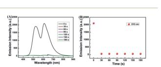
Fig. 5 (A) Time-dependent fluorescence intensity changes of sensor  $1-Cu^{2+}$  to  $H_2S$  in  $CH_3CN-H_2O$  (7/3, v/v) solution. (B) Relative fluorescence intensity at 610 nm as a function of time in  $CH_3CN-H_2O$  (7/3, v/v) solution.
