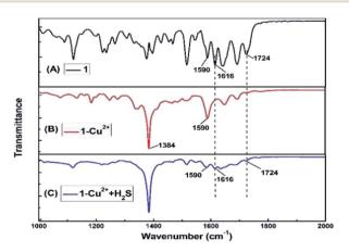
Fig. 8 Partial FT-IR spectra of 1 (A),  $1-Cu^{2+}$  (B) and  $1-Cu^{2+}+H_2S$  (C).
