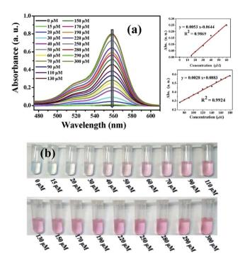
Fig. 6 (a) Absorption intensity of probe solution with various concentrations of PA (left) and linear fitting curve of the absorption intensity at 560 nm *versus* the concentration of PA (right); (b) color changes of the probe solutions with gradually addition of PA under visible light.
