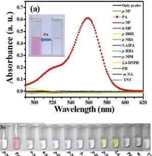
Fig. 3 (a) Absorption spectra of L (20  $\mu$ M) in the presence of various phenols (200  $\mu$ M) or NCAs (200  $\mu$ M); (b) corresponding photographs.
