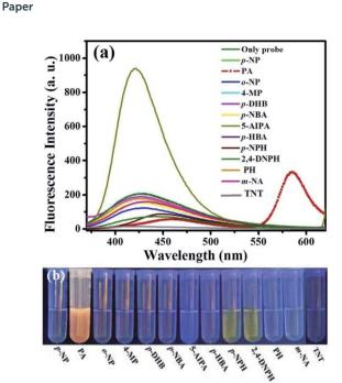
Fig. 4 (a) Fluorescence spectra of L (20  $\mu$ M) in the absence and presence of 200  $\mu$ M various aromatic compounds ( $\lambda_{ex}=314$  nm, slits: 2.5 nm/5 nm; slits: 1.0 nm/5 nm for 5-AlPA); (b) photograph of probe solutions with different aromatic compounds under 365 nm UV lamp.
