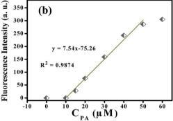
Fig. 7 (a) Fluorescence response of L (20  $\mu$ M) upon addition of PA from 10 to150  $\mu$ M (inset, the proposed structure of the spiro-lactam ring-opening product); (b) linear fitting analysis ( $\lambda_{ex}=314$  nm,  $\lambda_{em}=586$  nm) of the fluorescence intensity at 586 nm *versus* the concentration of PA.
