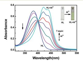
Fig. 2 The changes in absorption spectra and color of HL induced by  $Al^{3+}$  in acetonitrile (2.0  $\times$  10<sup>-5</sup> mol L<sup>-1</sup>).
