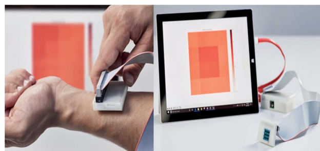
Fig. 15 sKan device. This device detects skin cancer using thermal images that are obtained from affected areas of the skin surface using thermistors. Reproduced from ref. 202.
