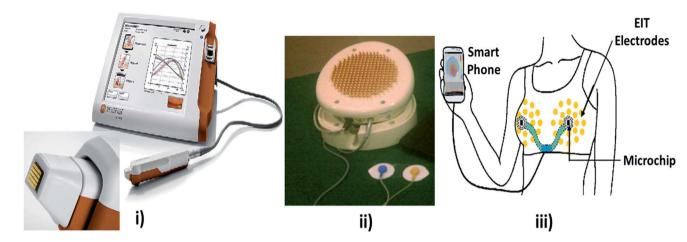
Fig. 16 Electrical bio-impedance measurement setup. In the above image shown (i) Nevisense device including hand piece and touch screen monitor. (Courtesy of SciBase, Stockholm, Sweden; with permission); (ii) Electrical impedance mammograph meik, reproduced under CC license from ref. 227; (iii) Smart phone based diagnosis using EIT patch.
