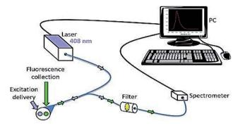
Fig. 10 Fluorescence spectroscopy. It is used to detect the skin cancer with the help of fluorophores. Reprinted from ref. 145 with permission from Elsevier.
