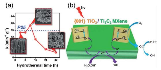
Fig. 4 (a) Photocatalytic degradation rate constant (k) of (001)TiO<sub>2</sub>/Ti<sub>3</sub>C<sub>2</sub> prepared for different hydrothermal times. (b) Schematic illustration of the charge-transfer process over (001)TiO<sub>2</sub>/Ti<sub>3</sub>C<sub>2</sub>. Reprinted from ref. 56 with permission. Copyright 2016 American Chemical Society.
