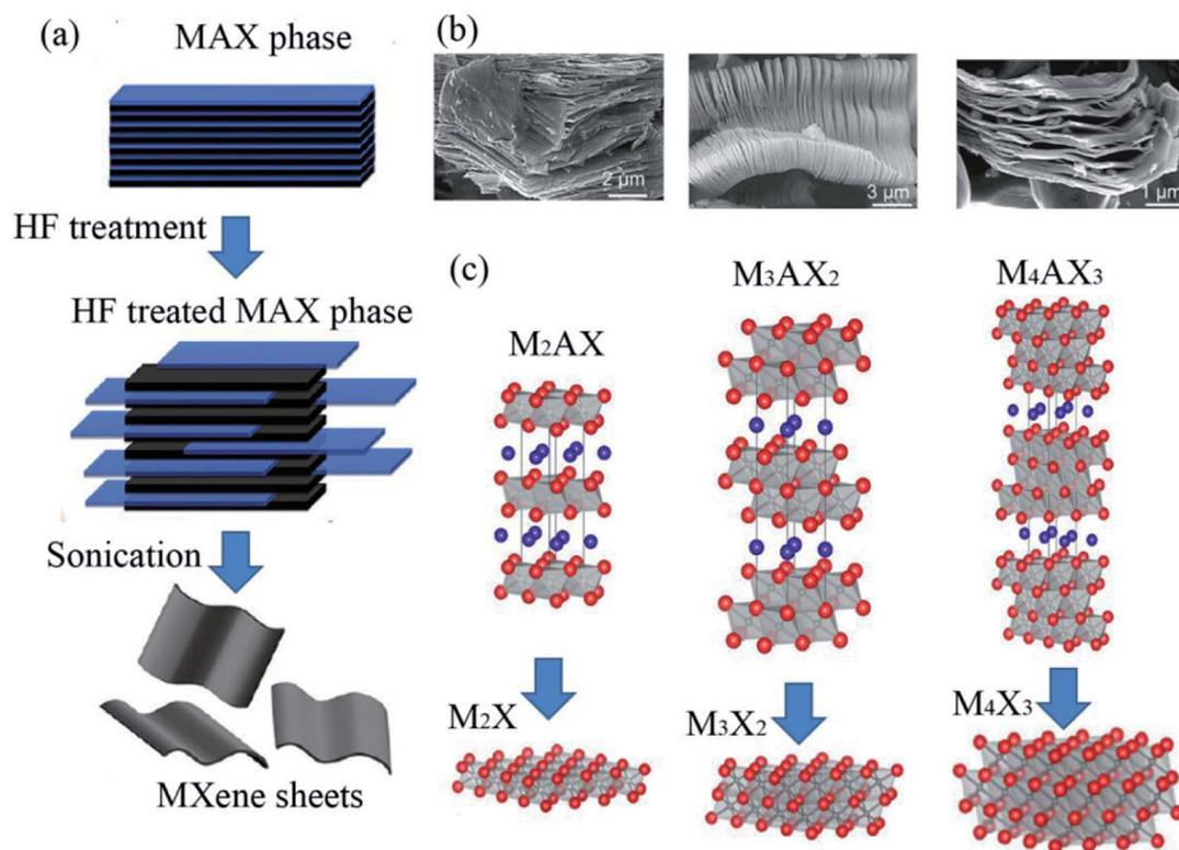
Fig. 1 (a) Early reported three different structures of MXenes (non-terminated):  $M_2X$ ,  $M_3X_2$  and  $M_4X_3$ . Reprinted from ref. 22 and 23 with permission. (b) SEM images of  $Ti_2AlC$ ,  $Ti_3AlC_2$  and  $Ta_4AlC_3$  after HF treatment (from right to left). (c) Schematic illustration of the synthesis of MXenes from MAX phases. Copyright 2013 John Wiley and Sons and Copyright 2012 American Chemical Society.
