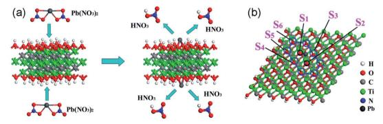
Fig. 3 (a) Schematic illustration of the formation of the  $Ti_3C_2(O_2H_{2-2m}Pb_m)$  structure from  $Ti_3C_2(OH)_2$  to  $Ti_3C_2(O_2H_{2-2m}Pb_m)$ ; (b) top-view of the  $Ti_3C_2(O_2H_{2-2m}Pb_m)$  structure when the Pb coverage is 1/9 ML. S1-S6 represent the different atom sites of the hydroxyl. Reprinted from ref. 44 with permission. Copyright 2015 American Chemical Society.
