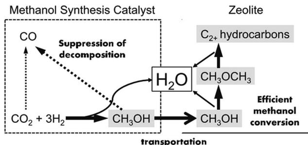
Fig. 11 Reaction steps of CO<sub>2</sub> hydrogenation over composite catalyst (favorable paths are shown in bold lines). Reprinted with permission from ref. 125. Copyright 2015 Elsevier.
