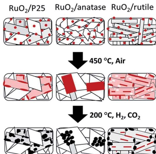
Fig. 5 Schematic illustration of the shape evolution of  $\text{RuO}_2/\text{TiO}_2$  catalysts: after  $\text{RuO}_2$  nanoparticle deposition, after thermal annealing at  $450^\circ\text{C}$ , and after reduction and methanation. Red indicates  $\text{RuO}_2$ , pink indicates thin  $\text{RuO}_2$  layer, white indicates Ru depleted area, and black indicates metallic Ru. Reprinted with permission from ref. 67. Copyright 2013 RSC.
