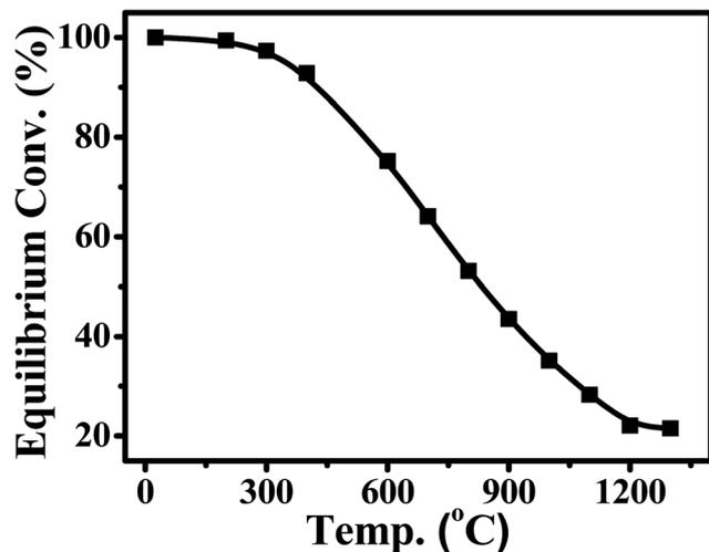
Fig. 3 Equilibrium conversion of CO<sub>2</sub> in methanation at different temperatures (plotted using the data from the literature).<sup>39,40</sup>
