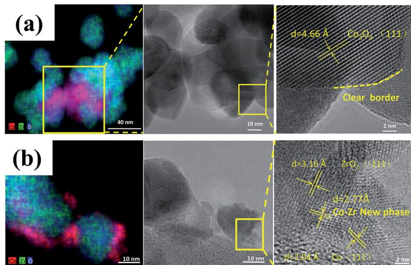
Fig. 4 STEM-EDS maps and corresponding TEM images of (a) calcined catalyst precursors  $\text{Co}_3\text{O}_4/\text{ZrO}_2$  and (b) reduced catalyst  $\text{Co}/\text{ZrO}_2$ . Reprinted with permission from ref. 62. Copyright 2017 Elsevier.
