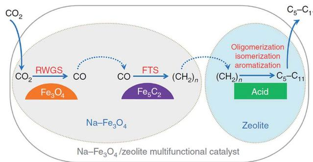
Fig. 9 Reaction scheme for CO<sub>2</sub> hydrogenation to gasoline-range hydrocarbons through modified FTS route. Reprinted with permission from ref. 105. Copyright 2017 Nature.
