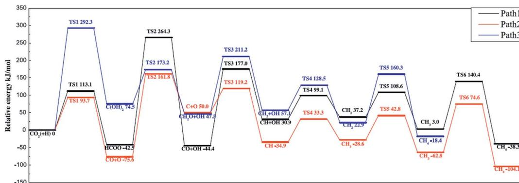
Fig. 7 Potential energy diagram of three mechanisms of CO<sub>2</sub> methanation. Reprinted with permission from ref. 92. Copyright 2015 Elsevier.
