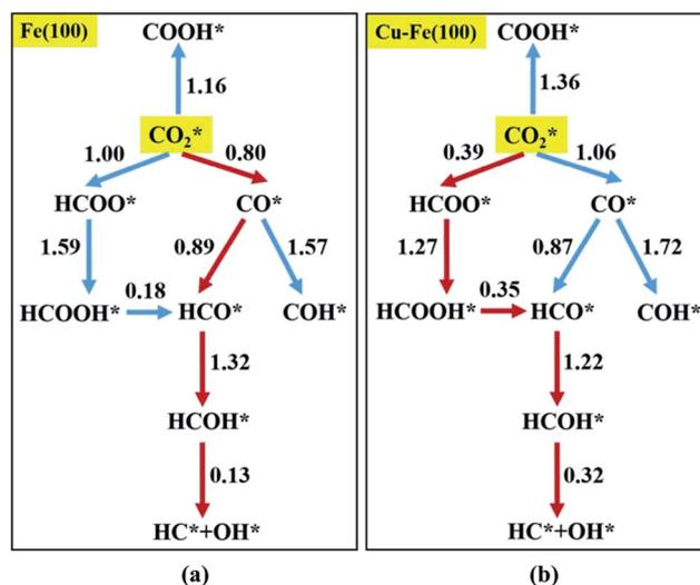
Fig. 12 Reaction networks examined to identify energetically favorable C1 species from CO<sub>2</sub> hydrogenation on (a) Fe(100) and (b) Cu–Fe(100) surface at 4/9 ML Cu coverage. Activation barriers are given in eV (the networks connected with red arrows represent the preferred path for CO<sub>2</sub> conversion to CH<sup>\*</sup>). Reprinted with permission from ref. 109. Copyright 2017 ACS.
