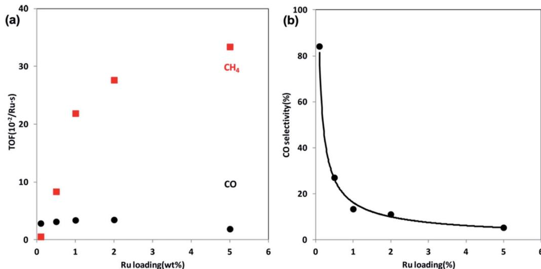
Fig. 6 (a) TOFs of CO and CH<sub>4</sub> formation at steady state at 300 °C over Ru/Al<sub>2</sub>O<sub>3</sub> catalysts as a function of Ru loading. (b) CO selectivity as a function of Ru loading at 300 °C. Reprinted with permission from ref. 47. Copyright 2013 ACS.
