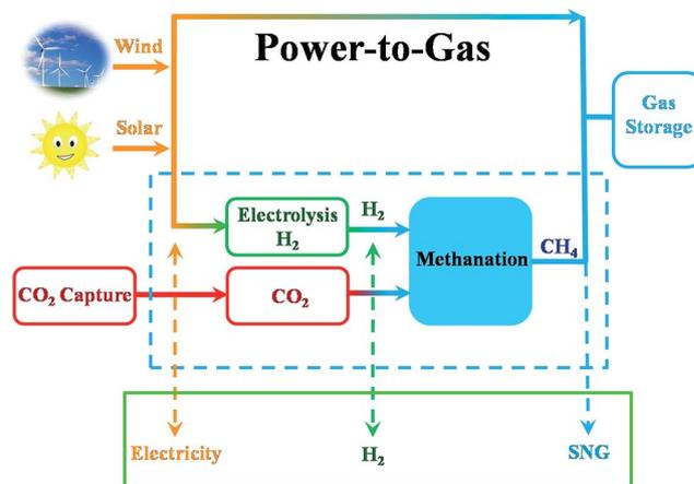
Fig. 2 Schematic illustration of CO<sub>2</sub>-based sustainable production of chemicals and fuels.
