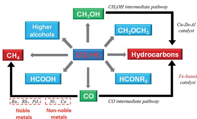
Fig. 1 Conversion of CO<sub>2</sub> to chemicals and fuels through hydrogenation.
