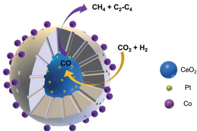
Fig. 10 Schematic diagram of CO<sub>2</sub> hydrogenation on CeO<sub>2</sub>–Pt@SiO<sub>2</sub>–Co core-shell catalysts. Reprinted with permission from ref. 118. Copyright 2017 ACS.
