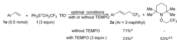
**Scheme 4** Evidence for the radical process. <sup>a</sup> The yield was determined by  $^{19}\text{F}$  NMR spectroscopy; <sup>b</sup> the yield was calculated based on TEMPO as the limiting reagent.
