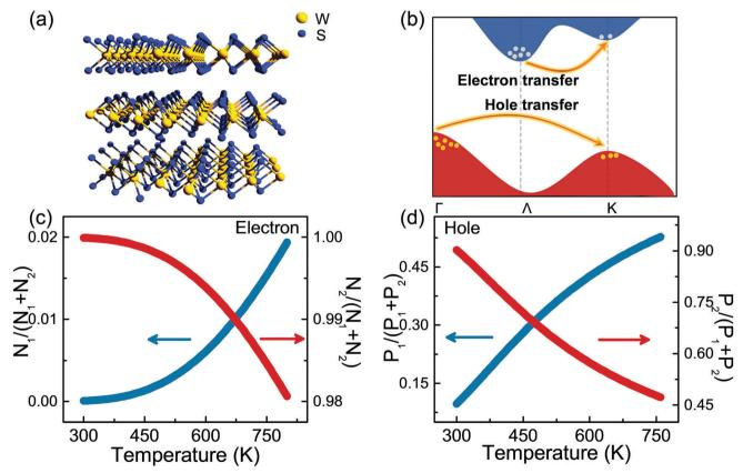
Fig. 1 (a) Structural schematic diagram of a multilayer 2H-WS<sub>2</sub> sample. (b) A scheme showing the transfer process of photo-carriers among different energy valleys and hills; the orange arrows indicate the transfer direction from  $\Lambda/\Gamma$  to K. Population ratio of the electrons (c) and holes (d) in the K point (blue curve) and the  $\Lambda/\Gamma$  point (red curve) as a function of the measurement temperature in ML-WS<sub>2</sub>.
