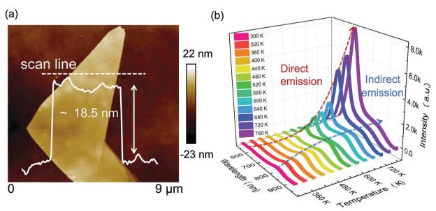
Fig. 2 (a) A typical AFM image showing the height profile of the mechanically exfoliated ML-WS<sub>2</sub> flake. (b) Steady-state TD-PL spectra of the ML-WS<sub>2</sub> sample taken at a temperature range of 300-760 K; the red and blue dashed arrows respectively indicate the variations of direct and indirect emission peaks with temperature
