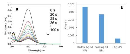
Fig. 16 (a) Time-dependent UV-vis absorption spectra of the catalytic reduction of 4-nitrophenol to 4-aminophenol by an excess amount of NaBH<sub>4</sub> by hollow Ag-Pd NPs synthesised in 3 CFI reactors connected in series, using Pd(NO<sub>3</sub>)<sub>2</sub> as precursor. (b) Average kinetic constant ( $K_{\rm app}$ ) value of hollow alloy Ag-Pd, solid alloy Ag-Pd (synthesised by simultaneous reduction with HQ) and Ag NPs (seeds).
