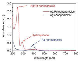
Fig. 3 UV-vis spectra of Ag nanoparticles formed after Reactor 2 and Ag-Pd bimetallic nanoparticles formed in Reactor 3 using  $K_2$ PdCl<sub>4</sub> as precursor.
