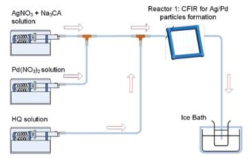
Fig. 11 Simultaneous reduction of  $Aq(NO_3)$  and  $Pd(NO_3)_2$  with HQ in a CFI microreactor.
