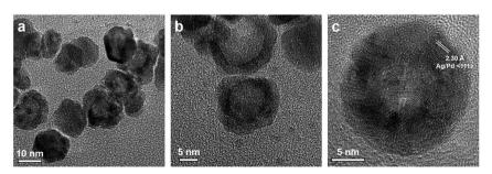
Fig. 6 (a–c) TEM and HTEM images of Ag–Pd hollow NPs (after Reactor 3) synthesised using  $Pd(NO_3)_2$  as precursor.
