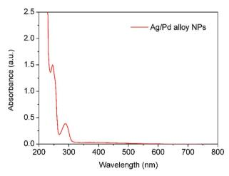
Fig. 12 UV-vis spectrum of Ag–Pd alloy NPs synthesized by simultaneous reduction of  $Ag(NO_3)$  and  $Pd(NO_3)_2$  with HQ. The solution was diluted for 10 times prior to characterisation.
