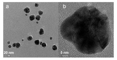
Fig. 13 (a) TEM and (b) HRTEM image for Ag-Pd alloy NPs synthesized by simultaneous reduction of  $Aq(NO_3)$  and  $Pd(NO_3)_2$  with HQ.
