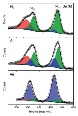
Fig. 3 Sn 3d XPS spectra of samples synthesized under  $H_2/N_2$ , Ar or air. Peak deconvolution shown corresponding to  $\mathrm{Sn}^0$  (green),  $\mathrm{Sn}^{\mathrm{IV}}$  (blue), and metallic Sn  $\mathrm{3d}_{3/2}$  (red).
