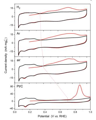
Fig. 6 CO stripping voltammograms of the as-prepared PtSn nanoparticles and commercial Pt/C (20 wt%, JM). A monolayer of CO is absorbed at 0.2 V vs. RHE. The first cycles, starting at 0.2 V, are shown in red and the third cycle is shown in black. Measurements were carried out in 1 mol dm $^{-3}$  H<sub>2</sub>SO<sub>4</sub> at 25 °C with a scan rate of 20 mV s $^{-1}$ . The onset potentials of CO oxidation as defined in the text are marked by red bars.
