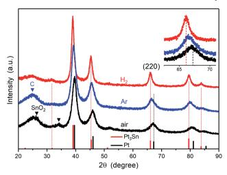
Fig. 2 XRD patterns of  $Pt_3Sn$  nanoparticles annealed under  $H_2$ , Ar and air. The inset shows the magnified region of the (220) peak. The standard patterns of  $Pt_3Sn$  (35-1360) and Pt (04-0802) were obtained from the JCPDS database.
