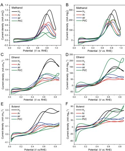
Fig. 7 Cyclic voltammograms illustrating the specific activities (A, C and E) and mass activities (B, D and E) of the heat treated Pt $_3$ Sn catalysts and the commercial Pt/C reference catalyst in 0.1 mol dm $^{-3}$  H $_2$ SO $_4$  and 0.1 mol dm $^{-3}$  (A and B) methanol, (C and D) ethanol, and (E and F) 1-butanol at 25 °C with a scan rate of 50 mV s $^{-1}$ .
