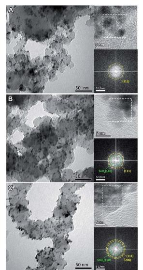
Fig. 1 TEM images of  $Pt_3Sn$  nanoparticles annealed under (A)  $H_2$ , (B) Ar and (C) air. The upper insets are the corresponding HRTEM images and the bottom insets are the fast-Fourier transform patterns on the selected area (white dashed square) in the corresponding HRTEM images. The dashed rings are drawn to connect bright spots at the same distance to the centre and represent the lattice fringes of the selected areas.
