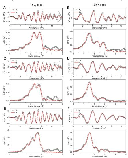
Fig. 5  $k^2$ -Weighted EXAFS spectra and their Fourier transforms (not phase corrected) of (A and B) Pt<sub>3</sub>Sn NPs annealed under H<sub>2</sub>, (C and D) Ar, and (E and F) air. Spectra at the Pt L<sub>3</sub>-edge and Sn K-edge are on the left and right column, respectively. The data points and the fittings are plotted as empty dots and red lines, respectively.
