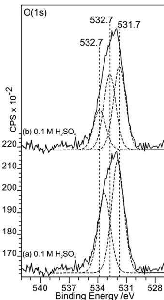
**Fig. 11** A comparison of curve fits of the O(1s) spectra from Fig. 8. In (a) and (b), fits to the acid treated surface spectrum using two and three components respectively are compared. Whilst two components are sufficient to fit the overall envelope, three components, in which a peak at 532.7 eV can be assigned to OH(a), is also successful. The three peak fit is consistent with a model in which OH(a) reduces Au<sup>3+</sup> to Au<sup>0</sup> showing that both produce acceptable models.
