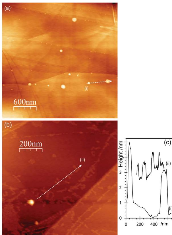
Fig. 8 AFM images of HOPG surfaces treated with aqua regia (AQR,  $3\text{HCl} : 1\text{HNO}_3$ ) and subsequently with a  $2 \times 10^{-6}$  M aqueous solution of  $\text{HAuCl}_4$ . (a) After treatment with 0.25 M AQR (b) after treatment with 1 M AQR followed by  $2 \times 10^{-6}$  M  $\text{HAuCl}_4$ ; (c) line profiles from (a) and (b) as labelled on the figure.
