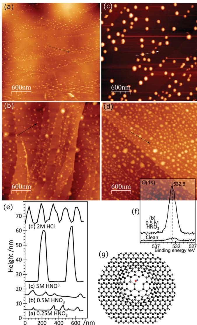
**Fig. 1** AFM images showing the effect of different acid treatments on HOPG surfaces: (a) 0.25 M HNO<sub>3</sub>; (b) 0.5 M HNO<sub>3</sub>; (c) 5.0 M HNO<sub>3</sub>; (d) 2.0 M HCl; (e) corresponding line profiles; (f) XP spectrum of (1s) region from image (b); (g) model previously proposed<sup>7</sup> to account for AFM features in which functionalisation of existing defects in the lattice leads to a local delamination.
