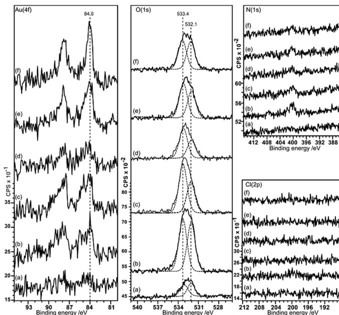
Fig. 5 XPS spectra showing the deposition of gold from a  $2 \times 10^{-6}$  M aqueous solution of  $\text{HAuCl}_4$  on HOPG surfaces pre-treated with  $\text{HNO}_3$  at different concentrations: (a) clean surface treated with gold solution; (b) 0.25 M  $\text{HNO}_3$ ; (c) 0.5 M  $\text{HNO}_3$ ; (d) 1.0 M  $\text{HNO}_3$ ; (e) 2.0 M  $\text{HNO}_3$ ; (f) 5.0 M  $\text{HNO}_3$ . Curve fitting of the spectra is discussed in the Experimental section.
