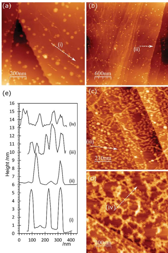
Fig. 4 AFM images of HOPG surfaces treated with HCl and subsequently with a  $2 \times 10^{-6}$  M aqueous solution of HAuCl<sub>4</sub>. (a) After treatment with 1 M HCl; (b) 0.5 M HCl followed by  $2 \times 10^{-6}$  M HAuCl<sub>4</sub>; (c) 1.0 M HCl followed by  $2 \times 10^{-6}$  M HAuCl<sub>4</sub>; (d) 1.0 M HCl, heated to 373 K followed by  $2 \times 10^{-6}$  M HAuCl<sub>4</sub>; (e) line profiles from (a–d) as numbered on figures.
