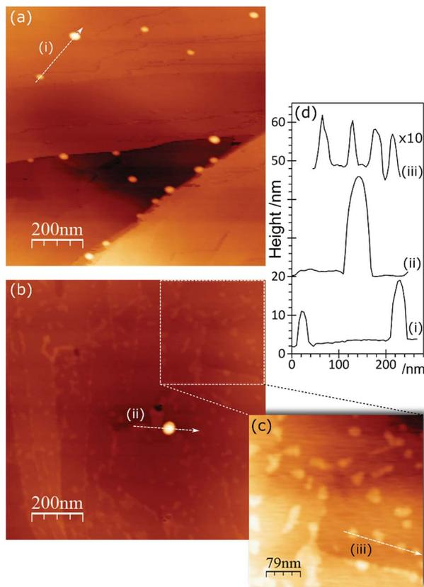
Fig. 10 AFM images of HOPG surfaces treated with  $\text{H}_2\text{SO}_4$  and subsequently with a  $2 \times 10^{-6}$  M aqueous solution of  $\text{HAuCl}_4$ . (a) After treatment with 0.1 M  $\text{H}_2\text{SO}_4$ ; (b) 0.1 M  $\text{H}_2\text{SO}_4$  followed by  $2 \times 10^{-6}$  M  $\text{HAuCl}_4$ ; (c) expanded section of (b). (d) Line profiles from (a)–(c).
