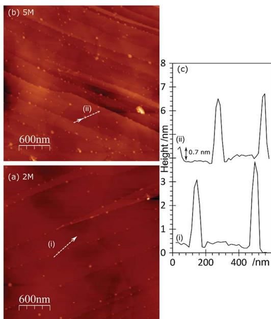
Fig. 6 AFM images of HOPG surfaces treated with HNO<sub>3</sub> and subsequently with a  $2 \times 10^{-6}$  M aqueous solution of HAuCl<sub>4</sub>. (a) After treatment with 2 M HNO<sub>3</sub> followed by  $2 \times 10^{-6}$  M HAuCl<sub>4</sub>; (b) after treatment with 5 M HNO<sub>3</sub> followed by  $2 \times 10^{-6}$  M HAuCl<sub>4</sub>; (c) line profiles from (a) and (b) as labelled on the figure.
