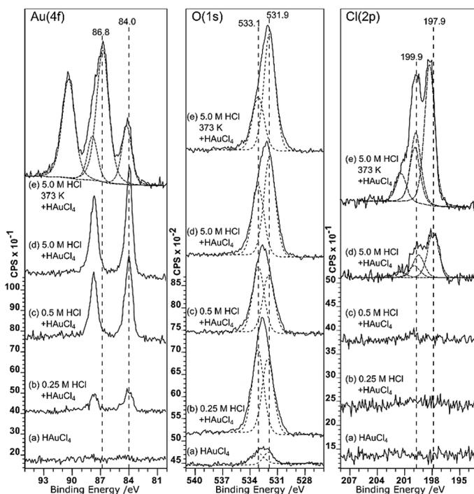
Fig. 3 (a)–(d) XPS spectra of HOPG samples pre-treated with HCl at different concentrations and then, after drying, to a  $2 \times 10^{-6}$  M aqueous solution of  $\text{HAuCl}_4$ . (e) Similar to (d) but heated to 373 K after treatment with HCl and then, after cooling to  $\sim 285$  K, treated with the  $2 \times 10^{-6}$  M  $\text{HAuCl}_4$  aqueous solution. Curve fitting of the spectra is discussed in the Experimental section.
