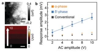
Fig. 5 PFM characteristics of various nanowire phases. (a) Height (above) and amplitude (below) mapping of the template's top surface filled with  $\delta'$ -phase nanowires. (b) Piezoelectric response amplitude of  $\alpha$ -phase (orange),  $\delta'$ -phase (blue) and conventional (black) nanowires as a function of AC amplitude.
