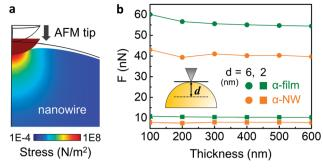
Fig. 4 Numerical simulation results of nano-indentation: (a) crosssectional view of a 6 nm indentation of a nanowire using a 25 nm AFM tip. (b) Indentation force change as a function of thickness of the film (green) and the nanowire (orange). The simulation was conducted using deformation depth (d) of 6 nm (circle) and 2 nm (square).
