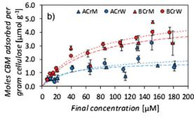
Fig. 3 (a) Methylene blue adsorption isotherms on regenerated cellulose scaffolds, (b) ThCBM<sub>CBHI</sub> adsorption isotherms on regenerated cellulose scaffolds. Error bars  $\pm 1$  standard error. Whilst a greater surface area is accessible to methylene blue in  $\alpha$ -cellulose samples, a greater area is accessible to ThCBM<sub>CBHI</sub> in bacterial cellulose samples. Water regenerated samples have a greater accessible area in all cases.
