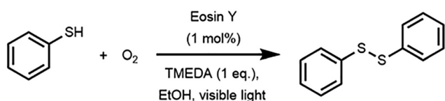
Scheme 1 Dimerization of thiophenol to diphenyl disulfide via photocatalytic aerobic oxidation with Eosin Y as photocatalyst.
