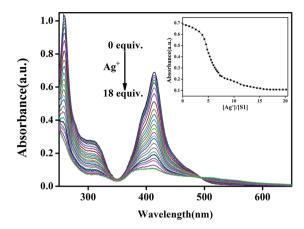
Fig. 4 Absorbance spectra of S1 (20  $\mu$ M) in the presence of different concentrations of Ag<sup>+</sup> (0–18 equiv.) in the DMSO/H<sub>2</sub>O (v:v = 1:1, buffered with HEPES pH = 7.2) solution. Inset: A plot of the variation in absorbance as a function of concentration of Ag<sup>+</sup> in the range from 0 to 18 equiv.
