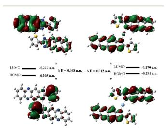
Fig. 7 DFT-optimized Frontier molecular orbitals and HOMO-LUMO energy gaps for **S1** (left) and **S1**-Ag<sup>+</sup> (right).
