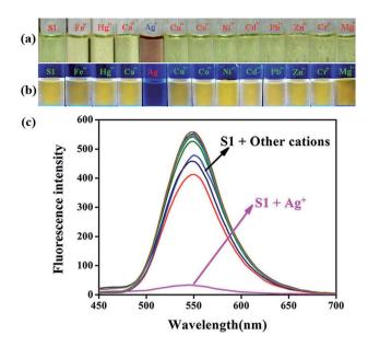
Fig. 1 An image of S1 upon the addition of 10 equiv. of various cations in DMSO/H<sub>2</sub>O (v:v = 1:1, buffered with HEPES pH = 7.2), which was taken under (a) visible light and (b) UV-lamp (365 nm) at room temperature. (c) Fluorescence spectral responses in DMSO/H<sub>2</sub>O (v:v = 1:1, buffered with HEPES pH = 7.2) of S1 (2.0  $\times$  10<sup>-5</sup> M) upon the addition of different cations (10 equiv.).
