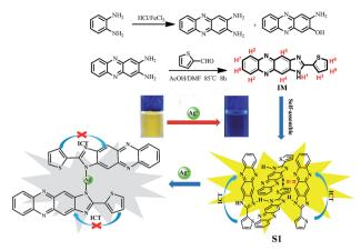
Scheme 1 Synthesis of the compound IM and the proposed possible mechanism of S1 bonding with Ag<sup>+</sup>.
