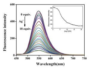
Fig. 3 Fluorescence spectra of S1 (20  $\mu$ M) in the presence of different concentrations of Ag $^+$  (0–18 equiv.) in DMSO/H $_2$ O (v:v = 1 : 1, buffered with HEPES pH = 7.2) solution. Inset: A plot of the fluorescence intensity depending on the concentration of Ag $^+$  in the range from 0 to 18 equiv.
