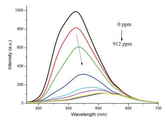
Fluorescence spectra of TBM-based film upon exposure to different amounts of TFA vapor ( $\lambda_{ex} = 420 \text{ nm}$ ).
