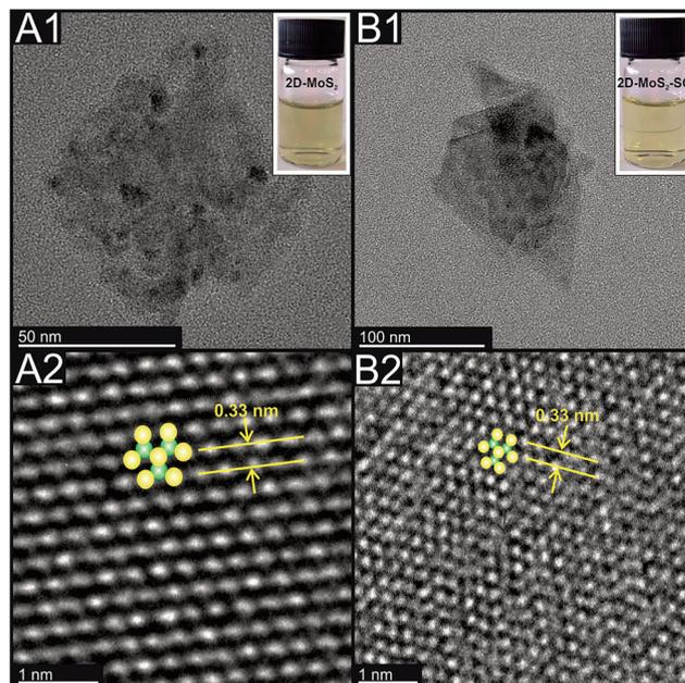
Fig. 1 TEM images of the commercially sourced 2D-MoS<sub>2</sub> (A1) scale bar: 50 nm; (A2) scale bar: 1 nm; and the exfoliated 2D-MoS<sub>2</sub>-SC (B1); scale bar: 100 nm, (B2); scale bar: 2 nm.
