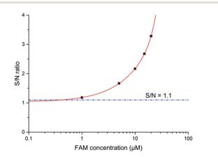
Fig. 9 S/N ratio as a function of concentration of FAM dye as OLEC driven at 20 V pulses. Solid red line predicted trends for the theoretical LOD at S/N = 1.1, which is shown with a dashed blue line.
