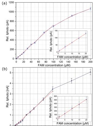
Fig. 8 Fluorescent detection measurement by integrated OLEC and OPD with different FAM dye concentration in water. The FAM solution was excited by the blue OLEC with brightness of (a)  $500 \text{ cd m}^{-2}$  and (b)  $2000 \text{ cd m}^{-2}$ ; the inset graph is the zoom-in of the low concentration part (1 to  $20 \mu \text{M}$ ).
