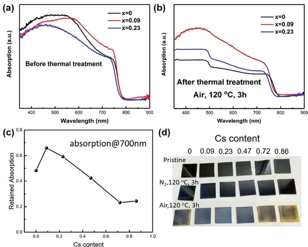
Fig. 1 Thermal stability study of perovskite films with different Cs content. (a) Perovskite films with compositions of  $\text{Cs}_x\text{MA}_{1-x}\text{PbI}_3$  before thermal treatment, where  $x$  represents Cs content. (b) Perovskite films after thermal treatment at 120 °C for 3 hours exposing to air. (c) Retained absorption at 700 nm for perovskite films with  $x$  ranging from 0 to 0.86. (d) Photographs of perovskite films exposing to different atmosphere.
