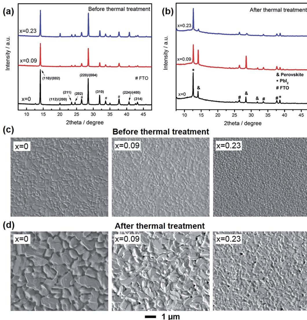
Fig. 2 Structure analysis of perovskite films. (a, b) XRD patterns for  $\text{Cs}_x\text{MA}_{1-x}\text{PbI}_3$  before and after thermal treatment. (c, d) Top-down view SEM images of perovskite films before and after thermal treatment.
