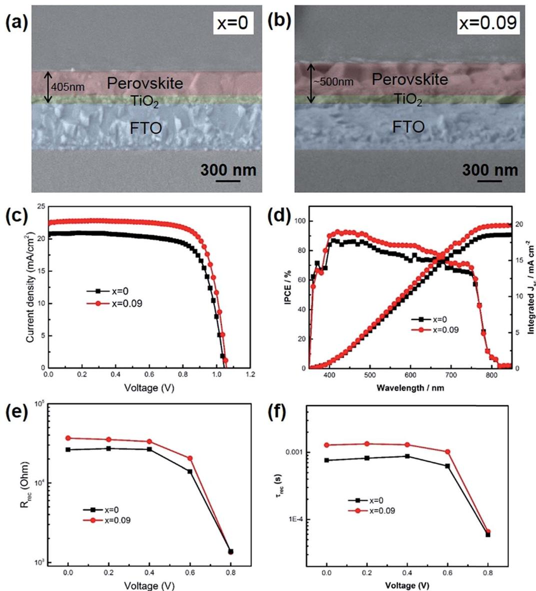
Fig. 3 (a, b) Cross-sectional SEM images of perovskite films with  $x = 0$  and  $0.09$ . (c)  $J$ - $V$  characteristics of champion devices with different Cs content. (d) IPCE and integrated photocurrent for the champion devices. (e) Recombination resistance derived from electrochemical impedance spectra (EIS). (f) Electron recombination time from EIS spectra.
