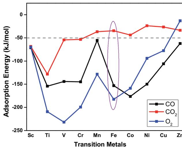
Fig. 2 Adsorption energies of CO (black), O<sub>2</sub> (blue) and CO<sub>2</sub> (red) on TM–PtSe<sub>2</sub> (TM = Sc–Zn).
