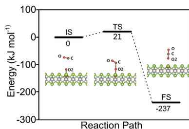
Fig. 7 Configurations of IS, TS and FS and energy profile along the MEP for CO reacting with O/Fe–PtSe<sub>2</sub>.
