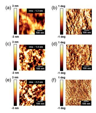
Fig. 3 AFM images of the pristine- [(a) and (b)], B- [(c) and (d)], and D-PEDOT:PSS films [(e) and (f)]. The left (a, c, e) and right (b, d, f) images are photographic and phase images, respectively. The concentrations of SDS used for blending and dipping methods were 40 and 100 mM, respectively. All images were obtained for an area of 250 nm  $\times$ 250 nm
