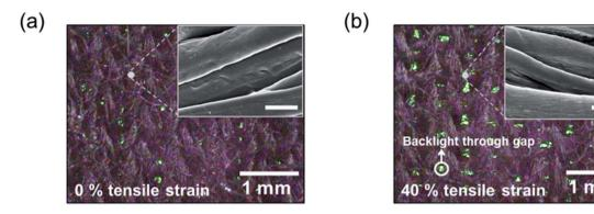
Fig. 6 Optical and SEM images of the BD-PEDOT: PSS-cotton before (a) and after (b) loading 40% tensile strain. The scale bar of the SEM image is  $10 \mu m$ .
