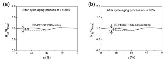
Fig. 8 The  $R_{\rm St}/R_{\rm 0,sat'}$  values of (a) BD-PEDOT:PSS-cotton and (b) BD-PEDOT:PSS-polyurethane during a cycle of 80% loading after performing the cycle-aging process at  $\varepsilon = 80\%$
