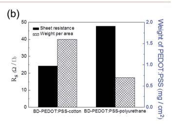
Fig. 4 (a) The highest conductivities of B-, D-, and BD-PEDOT:PSS films spin-coated on glass. (b) Sheet resistance (R<sub>S</sub>) and weight of PEDOT:PSS of BD-PEDOT:PSS-cotton and polyurethane.
