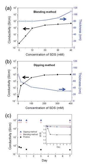
Fig. 1 Average conductivities and thickness of (a) B-PEDOT:PSS and (b) D-PEDOT:PSS. (c) Electrical stability tests of pristine-, B-, and D-PEDOT:PSS under constant conditions (relative humidity and temperature: 40% and 22.5 °C, respectively) for 7 days. The inset shows the normalised conductivity with respect to time.
