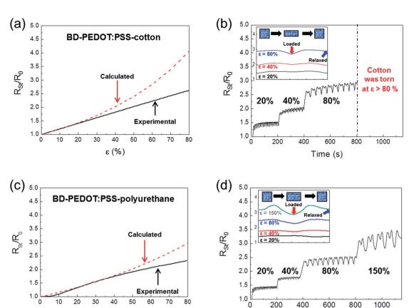
Fig. 5 Normalised resistance results of (a) BD-PEDOT:PSS-cotton and (c) BD-PEDOT:PSS-polyurethane with respect to tensile strain. The dotted and single curves correspond to the calculated and experimental data, respectively. Cyclic loading tests for (b) BD-PEDOT:PSS-cotton and (d) BD-PEDOT:PSS-polyurethane. The insets of (b) and (d) show changes in  $R_{St}/R_0$  during a cycle of ε-loading.
