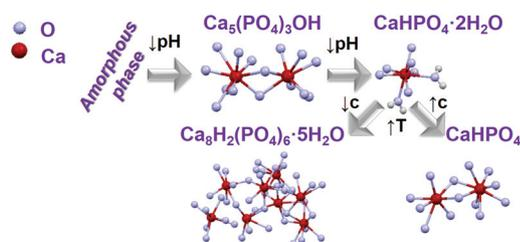
**Scheme 1** Schematic representation of transition between different calcium phosphate phases by changing synthesis parameters as pH, temperature (*T*) and concentration (*c*).<sup>11,16,37</sup>
