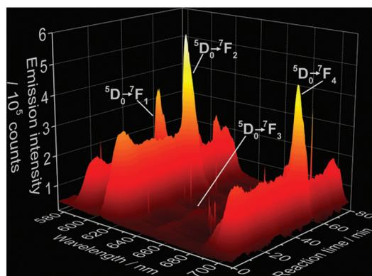
Fig. 2 Time-dependence of  $^5\text{D}_0 \rightarrow ^7\text{F}_J$  ( $J = 1–4$ ) electronic transitions of  $\text{Eu}^{3+}$  during the formation of doped calcium phosphate ( $\lambda_{\text{ex}} = 395\text{ nm}$ , experiment 5, Table 1). Sharper peaks parallel to the  $\text{Eu}^{3+}$  emission bands are assigned to measurement artifacts originated by the CCD detector.
