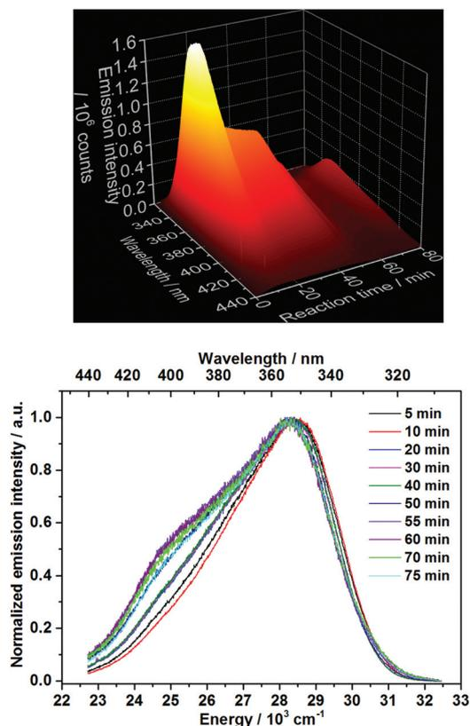
Fig. 1 Top: *In situ* emission spectrum recorded during calcium phosphate phase transitions applying 3% Ce<sup>3+</sup> as a coordination sensor ( $\lambda_{ex} = 280$  nm). Bottom: Normalized emission spectra for selected reaction times (experiment 2, Table 1).
