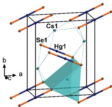
**Fig. 1** Fragment of the crystal structure of **1**, viewed approximately along  $\langle 00\bar{1} \rangle$ . The coordination polyhedron of one Cs atom is shown. All atoms are drawn with displacement ellipsoids at the 50% probability level.
