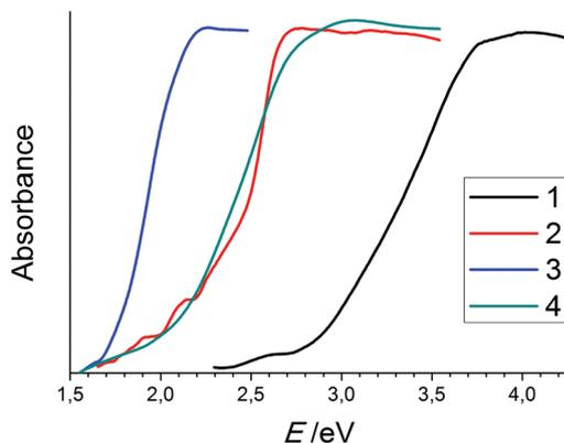
**Fig. 5** UV-Visible spectra of compounds 1–4. The following  $E_{\text{onset}}$  values were determined by means of the tangent method: 2.9 eV (1); 2.4 eV (2); 1.7 eV (3); 2.1 eV (4). Note that the onset of absorption for compound 2 is intrinsically red-shifted due to the beginning of decomposition of the very sensitive compound during sample preparation; for this, only the sharply ascending part of the curve was used to determine the optical gap.
