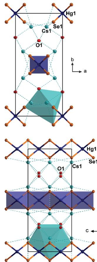
**Fig. 2** Fragments of the crystal structure of **2**, viewed along  $\langle 001 \rangle$  (top) and  $\langle 100 \rangle$  (bottom). The coordination polyhedra around the Hg atoms of the central strand and around one Cs atom are shown. All atoms are drawn with displacement ellipsoids at the 50% probability level.
